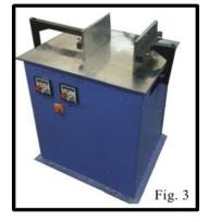
angles. The advantage of this machine over the earlier ones is that it can provide different phases of deformation to a single model at different angles of obliquity only by changing the ratio of speed of the moving pistons.
